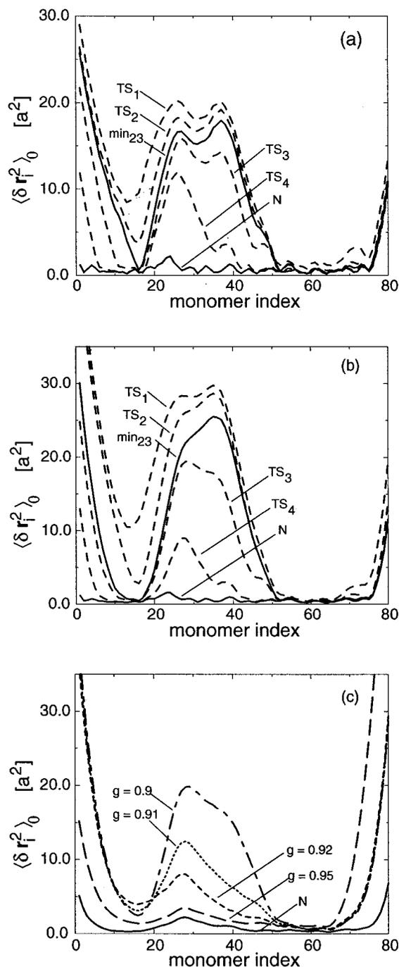
FIG. 9. Fluctuations vs sequence index  $\langle \delta r_i^2 \rangle_0 = G_{ii} a$  where  $a$  is the distance between successive monomers, of selected stationary points on the folding route for different persistence lengths. (a)  $l=2a$  ( $g=0.5$ ), (b)  $l=5a$  ( $g=0.8$ ), (c)  $l \approx 10, 11, 13, 20$  ( $g=0.9, 0.91, 0.92, 0.95$ ).
