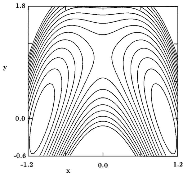
FIG. 4. Contours of the symmetric mode coupling (SMC) potential [Eq. (19)] for the parameters  $(\omega_x, \alpha) = (0.5, 1)$ . The interval of contours is 0.02 and the contours with the energy higher than 0.28 are omitted.
