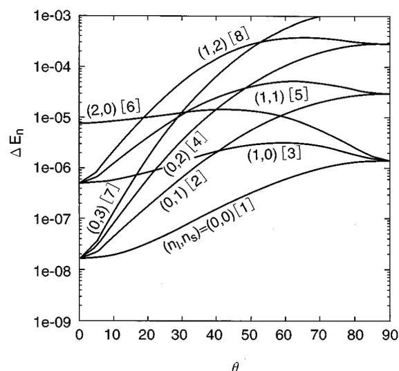
FIG. 6. Tunneling energy splitting (in logarithmic scale) of the V-parabola model (20) by the exact quantum mechanical calculation as a function of the coupling parameter  $\theta$ . Parameters  $(\omega_s, g)$  are equal to (0.7, 0.06).
